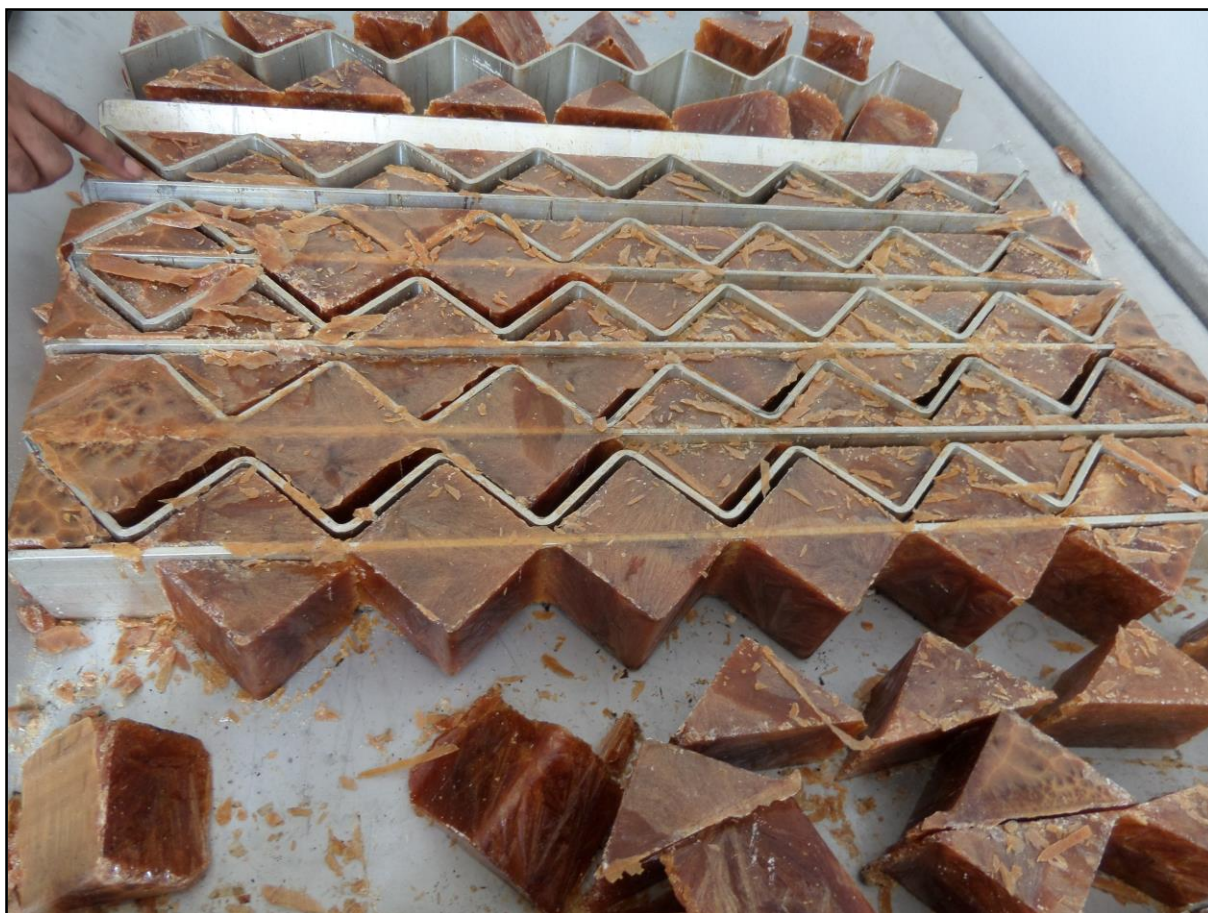
Portioning of explosives for reuse
